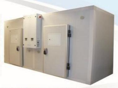
A refrigeration based de-Humidification system provided for avoid the condensation forming on test specimen as well as control the lower relative humidity.
